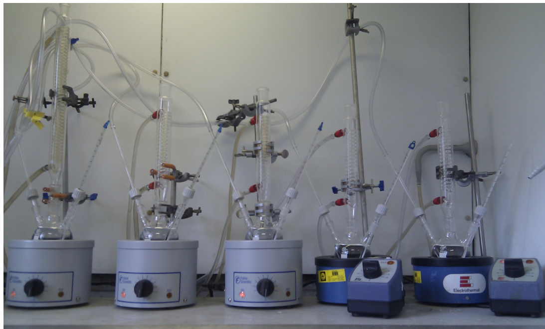
Figure 2.5: General setup of sandstone batch experiments.
